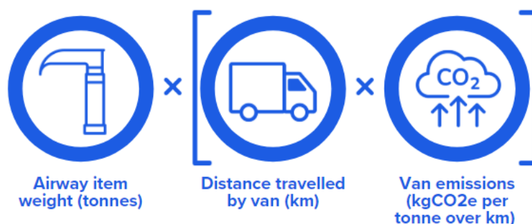
Figure 18: Calculation of carbon impacts for transport to disposal and off-site sterilisation (where applicable).
